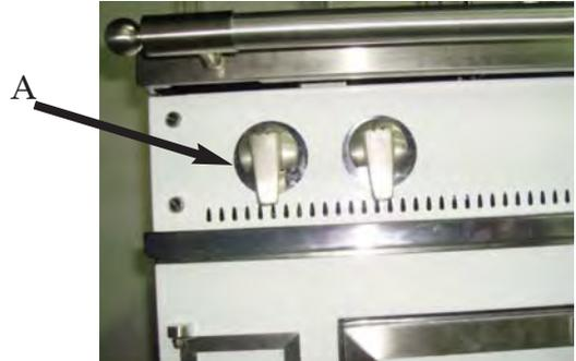
3. Rotate the by-pass screw on the valve body **to the left to increase** the flow rate, **to the right to reduce it**.
